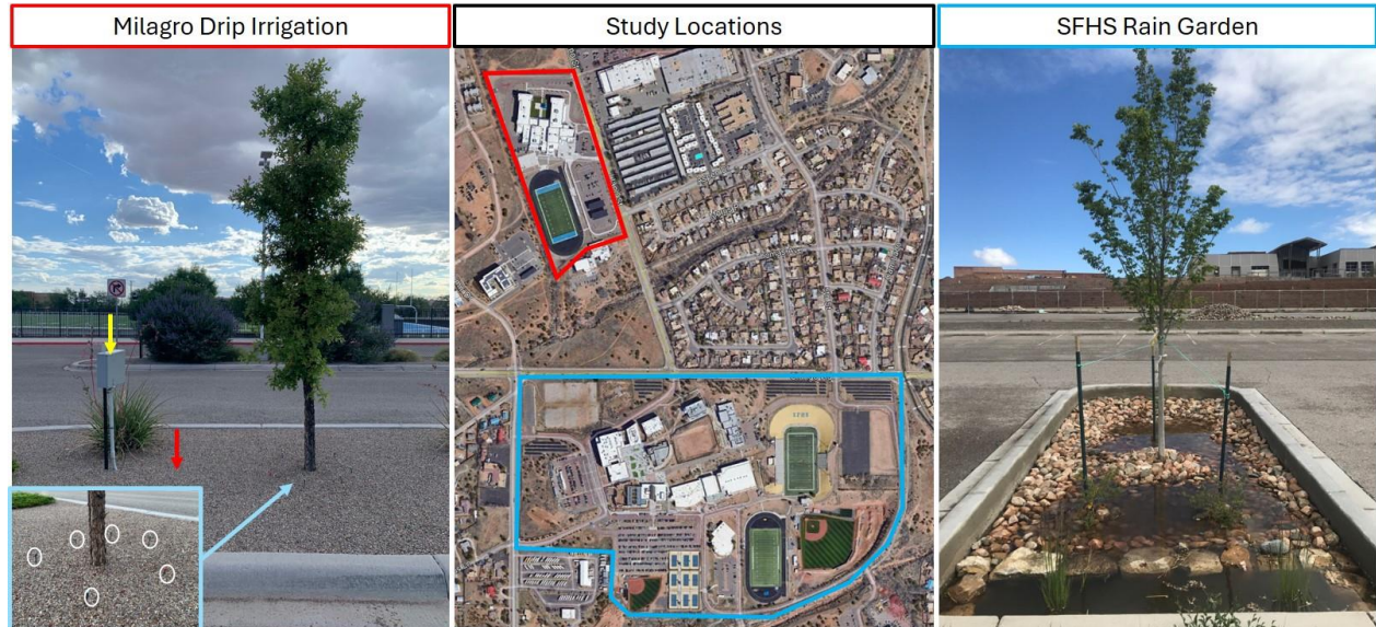
Figure 2. The campuses (center photo) of Milagro (red) and SFHS (blue) are located less than 0.5-miles apart. Example of a raised median (photo to left) with drip irrigation emitters (white circles) approximately 1ft from the root collar compared to a parking space retrofitted as a rain garden (photo to right) that is only irrigated during stormwater runoff from precipitation events. A soil moisture data logger (yellow arrow) and approximate location of subsurface VWC probes (red arrow) can be seen in the photo to the left.
