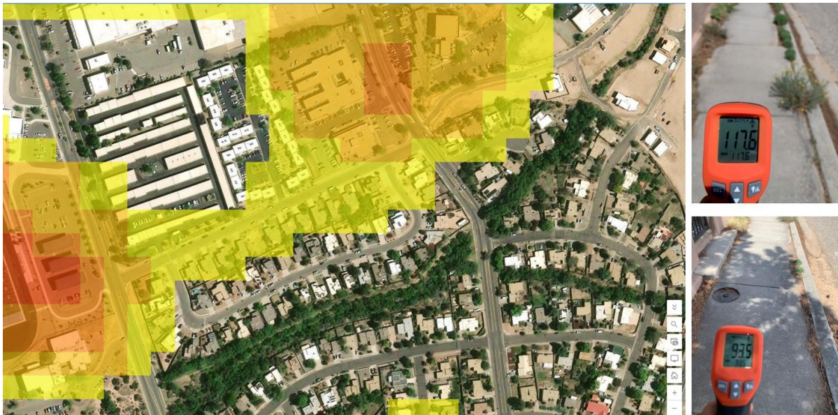
Figure 1. Urban heat island map (yellow, orange, red indicate increasingly hot temperatures) showing above-average surface temperatures resulting from impervious parking lots and dark rooftops compared to the shade canopy along an arroyo corridor in Santa Fe, NM (left). It is not uncommon for unshaded impervious surfaces (top right) to have temperatures substantially warmer than adjacent tree shaded surfaces (bottom right) by midday (117.6°F vs 93.5°F approx. 15ft apart). UHI map from ArcGIS and the Trust for Public Land.
