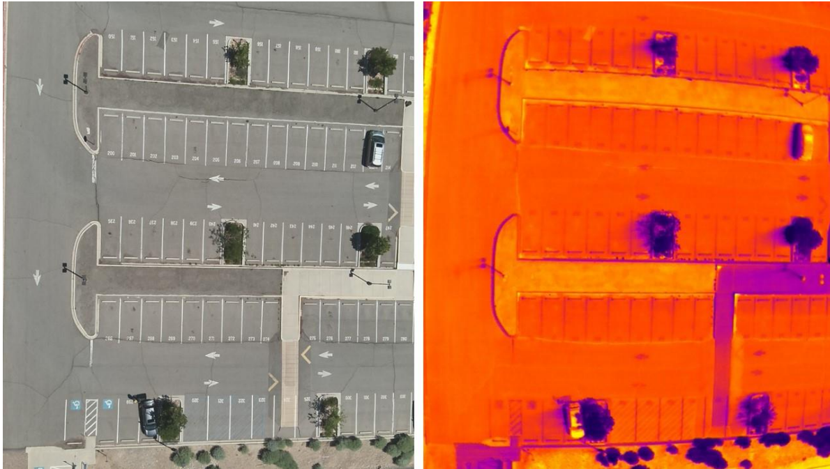
Figure 9. Conventional (left) and thermal (right) images of six rain gardens at SFHS taken at 11am in late July 2026 show the potential cooling value of trees and moist soils through evapotranspiration processes. The orange areas of asphalt were approximately 120°F while the shade under the trees (dark purple areas) was 89°F. Images courtesy of Tammy Huynh and Eva Schwendimann (Southwest Environmental Finance Center).
